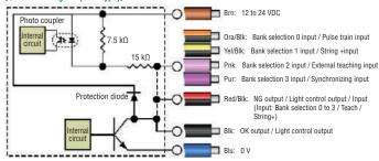
Typical example to connect Synchronous sensor, Rotary encoder, Reject mechanics and Bank-selection switch.
