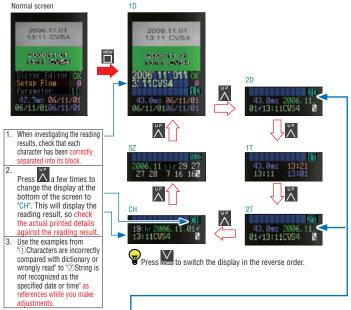
\* If the date or time has not been set, the character string is displayed, as shown here. The color of the characters indicates the match rate with the dictionary. If a character's offset from the dictionary exceeds the value set with [CharMrgn] (P.11), the character is displayed as a question mark ("P.11).
