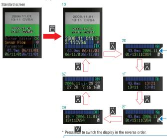
\* If the date or time has not been set, the character string is displayed, as shown here. The color of the characters indicates the match rate with the dictionary. If a character's offset from the dictionary exceeds the value set with [CharMrgn] (P.11), the character is displayed as a question mark ("?").
