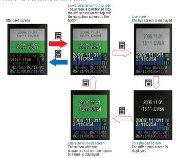
If you want to configure settings and perform teaching of the captured screen from, for example, the thresholded screen, press an on the thresholded screen to enable these operations while the thresholded screen is still displayed (you can return to the normal screen with the thresholded screen displayed).
