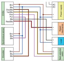
$<sup>^{\</sup>star}$  When capturing images of moving objects, timing input from a synchronous sensor is required.
