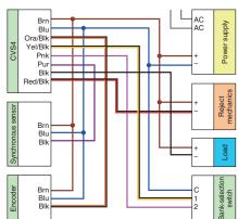
$<sup>^{\</sup>star}$  When capturing images of moving objects, timing input from a synchronous sensor is required.
