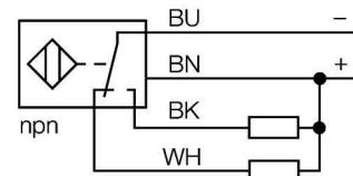
Inductive sensors detect metal objects contactless and wear-free. For this, they use a high-frequency electromagnetic AC field that interacts with the target. Inductive sensors generate this field via an RLC circuit with a ferrite coil.
